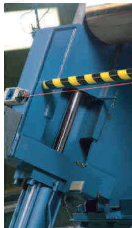
Pre-bending to the full rated capacity plate is accomplished with sufficient power in each side roll hydraulic cylinder. Many competitors are not capable of pre-bending to their maximum rated rolling capacity.
