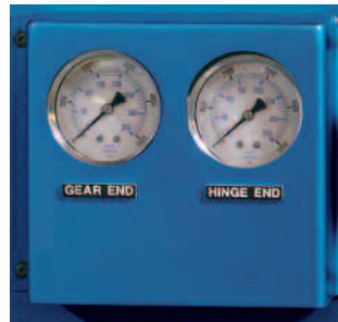
Pressure gauges monitor pinch pressure on both ends of the machine to monitor part squareness.
